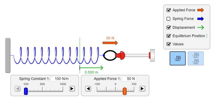
Check all five boxes on the right hand side (applied force (*F*), spring force, displacement ( $\Delta \ell$ ), equilibrium, values). Leave the blue slider control, which affects the spring constant, also sometimes called the constant of elasticity, but always abbreviated with k, always in the same value, for exemple 100 N/m. Play around with the red slider control for the applied force. Use only positive values.
