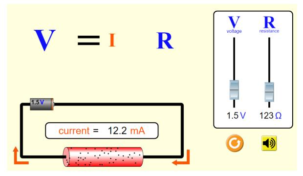
Leave Voltage Slider always in the same value, for exemple to 4.5 V and use the Resistance slider to set the Resistor to the values in the table.
