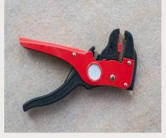
Device used to strip the electrical insulation from electric wires.
