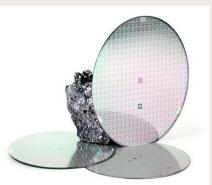
**Silicium** is a semiconductor element used in the construction of photovoltaic cells.
