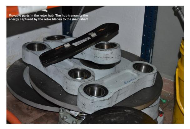
Movable parts in the rotor hub. The hub transmits the energy captured by the rotor blades to the main shaft. The hub is where the three blades are attached, which looks like an egg. It allows to transform the wind's linear kinetic energy to the rotational motion of the blades needed to turn the generator shaft.
