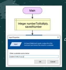
Let's read the value of the number to multiply. We insert an "Input instruction" by clicking on the arrow above the declaration box. We type the var name to read and press "OK"
