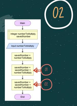
We insert 2 "Assign Instruction" to add "numberToMultiply" to "savedNumber" variable. By this way we have multiplied the initial number by 3.
