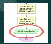
To display the result we add an output instruction, with the name of the variable "savedNumber"
