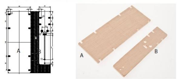
2. Mark and cut the cable channel with a craft knife or a chisel (B) between 4 mm hle and the sitch (Pattern broken line).
