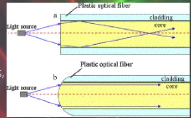
plastic optical fiber are used to get the light in a specific direction. In the end the photons are detected by photodetectors.
