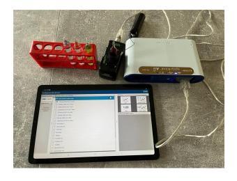
Sparklink – for measuring you'll need again chemicals and then tablet. When we have chnemicals, we connect Sparklink to the tablet (as you can see on photo) and add the chemicals in the black device. Then we cover the chemicals with black top (because it also, as the Colorimetr, uses light to measure, but kinda different) and find on tablet value, that we are measuring. Then we start measure.
