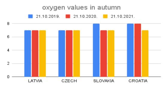
Graph 12 shows that the measured oxygen levels at the stations in Latvia and the Czech Republic are the same. As with graph 11, we see that in Slovakia and Croatia the amount of oxygen in the water is higher in 2019 and lower in 2021.
