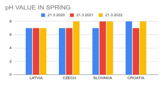
Graph 3 shows that the acidity of the water at the measuring stations is uniform, so our conclusion is that there is no influence of pollution. Natural waters have a pH of around 8, our measured values show more precipitation that reduces the acidity of the water, which is a characteristic of spring.
