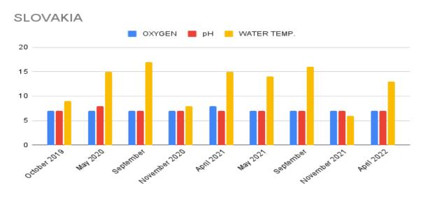
Graph 22: Values of measured oxygen, pH, water temperature at the measuring station in Slovakia.
