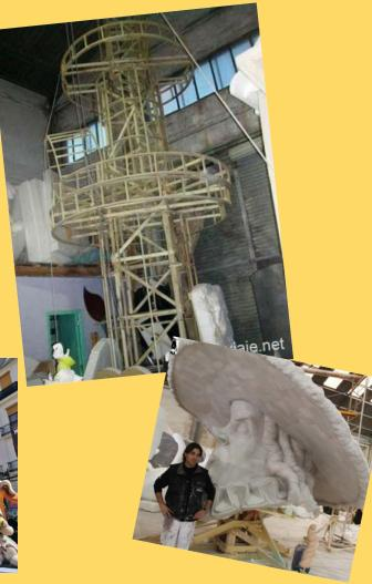
**3.** <u>**Construction with expanded polystyrene:**</u> It is the modern and the cheaper one. Each "ninot" is made directly on white polystyrene and then joined to the wood skeleton. They are polish to eliminate physical imperfections, then recovered with paper and glue and finally painted.
