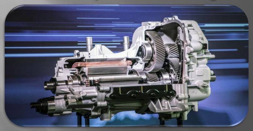
It develops 204 hp and launches Opel Ampera in transmission and differential transmission
