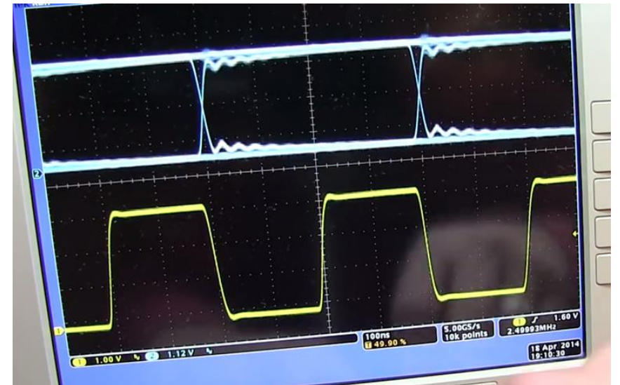
Eye pattern affected by noise and ISI
