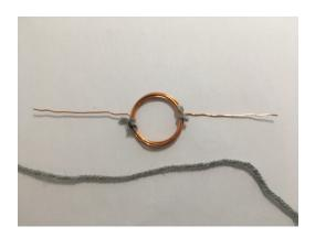
→ Now you need to fabricate the contacts. For this get a knife and scrape one side of the marked 5cm off completely and just half on the other. This is a really important step, if you do not do it right you will need to cut off an edge. The blue part in the following sketch is how you need to scrape off the insulation. Don't scrape off the orange part.
