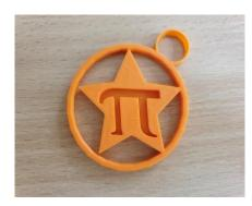
Students can create key rings in different shapes. The main parts of the pattern are the letter and the ring for fastening. Both of these parts are found in base forms. It teaches how to align two models with a special tool and combine them into one model. Advanced students can be given a
