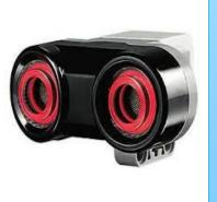
Ultrasonic Sensor for Obstacle Avoidance
