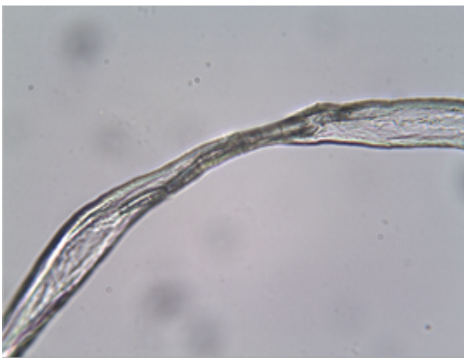
COTTON: fibres with smooth contours, with frequent
