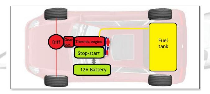
A stop-start hybrid is the simplest form of hybridization, if one wants to classify it as a "hybrid" at all, or merely an aid to efficiency.
