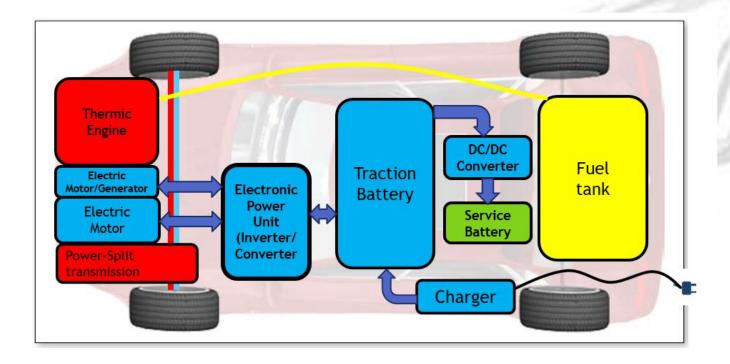
This hybrid cars drivetrains combine the serial and parallel systems.
