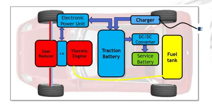
Parallel HEV drivetrain, allow the vehicle to be powered by both the electric motor and/or the internal combustion engine (separately or in combination).
