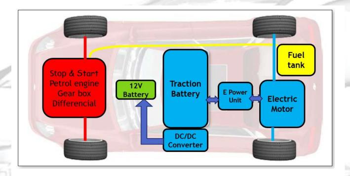
The thermic engine moves a rolling train (ex: front) while the electric engine moves another one (ex: rear).
