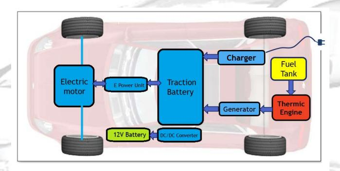
The serial HEV concept is characterized for the exclusive purpose of electric driving.
