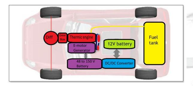
Mild hybrids are primarily powered by a gasoline engine and assisted by an electric motor, allowing the internal combustion engine to be turned off whenever the car is stopped, yet restarted quickly.
