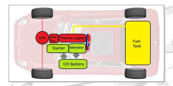
An internal combustion engine (ICE) is an engine where the combustion of a fuel (petrol or diesel) applies direct force to pistons of the engine.
