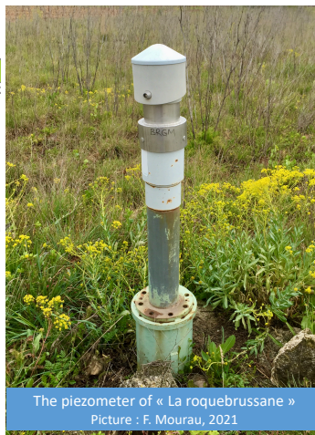
Figure 5: The piezometer is an instrument that measures the depth of the water table
