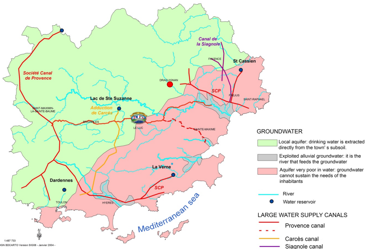
Figure 2 : Resources used for drinking water supply
