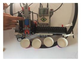
Students built "Colour Sorter with EV3" to scan and load coloured object and let them in the right area. The students saw that sensor data can control systems using feedback and understand ratio concepts and use ratio reasoning to solve problems. The Colour Sorter uses the Array functions to store and play back data. By storing the colour and place each colour tile, the robot can then sort the objects out mechanically.
