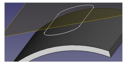
We could try to immediately use the protrusion tool but it will not work. FreeCAD don't allow multiple solid parts in the same document. So we first want to "fix" this sketch on the upper face of our solid base.
