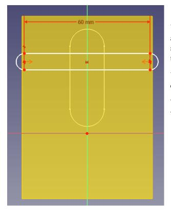
You know how it works now. By using the slot tool and some constraints (horizontal distance and symmetry) try to reproduce this sketch then click ok to leave the sketch.
