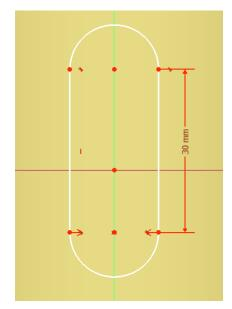
By using the predefined constraints of the slot tool try to draw something like this.
