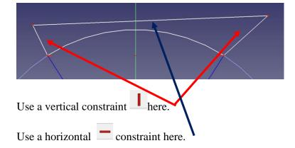
Give a height I of 10 mm to one of the vertical lines (no need to do it to both of them because we previously defined a symmetry constraint).
