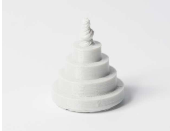
Figure 53: Print of vertical pins with decreasing diameter (from 25 to 5mm) illustrating the upper diameter of the print becoming too small to print accurately. [75]
