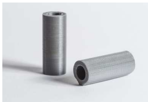
Figure 26: Quality differences in the same piece, according orientation. [38]
