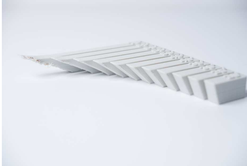
Figure 51: The effect of increasing overhang angle (in increments of 5 degrees) on print quality. Max. angle shown is 70 degrees. [73]
