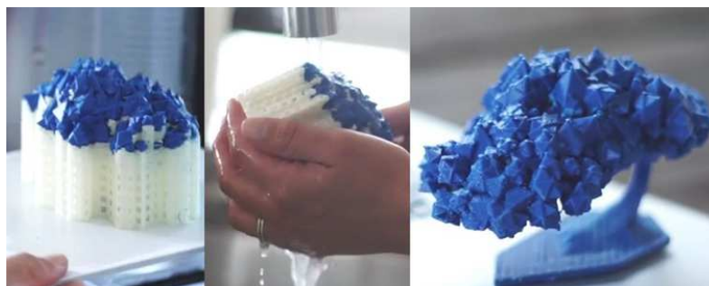
Figure 37: Bath for removing the support structures. [49]
