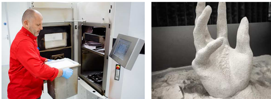
Figure 34: SLS extraction process. [46]
