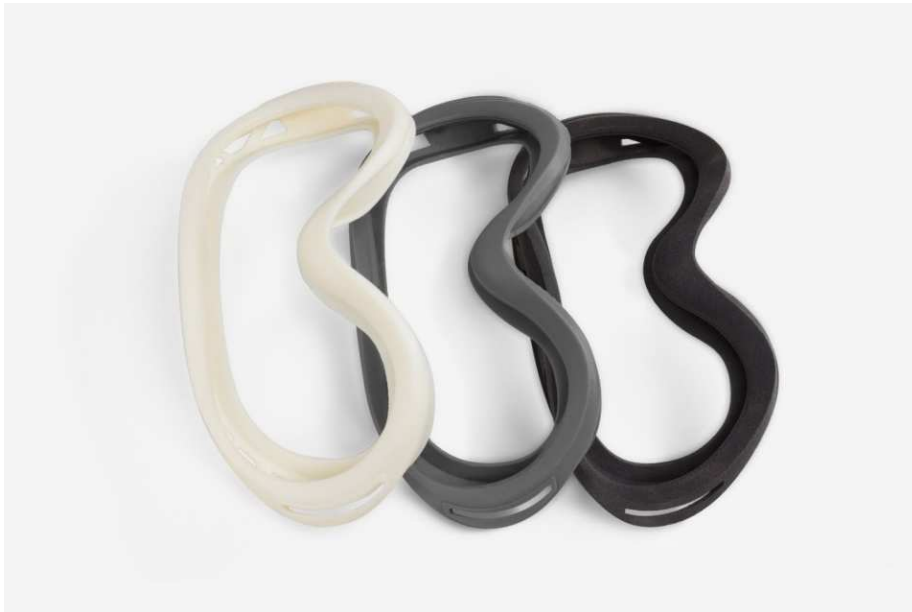
Figure 5: Prototypes of a ski goggles' frame printed with FDM, SLA and SLS technology (from left to right) [8]
