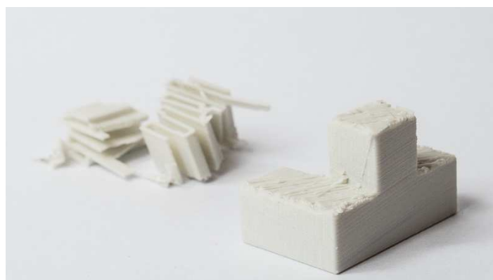
Figure 49: FDM printed puzzle piece with support removed showing surface roughness. [71]
