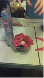
Results: On the first throw, the depth of the impact measured 0.5cm. When we placed the "astronaut suit" on the sand we noticed the impact's depth measured 0.2cm.
