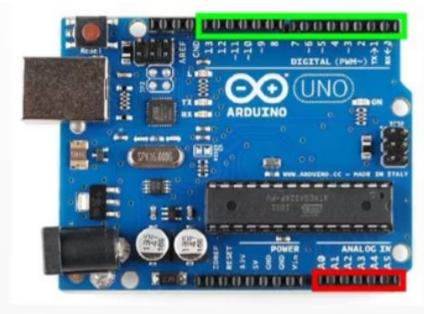
We could connect the following input / output pins.
