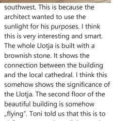
protect the first floor, where the entrance and a cafe are located, from too much sunlight or rain. The temperature inside of the building gets regulated through two steps: 1. Between the facade and the actual building is a hollow space. 2. There are pipes full of water, that can regulate the temperature, either to make it warm or cool.
