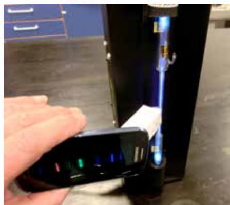
Using a foldable mini-spectrometer to obtain the helium emission spectrum
