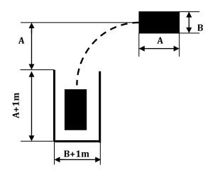
The car has to be parked from its starting position making one reverse motion as it is shown on the figure. When the vehicle is stationary its dimensions must be within the markings. The automobile should not touch the markers while entering (leaving) the parking place. Its wheels should not touch the markings, too.
