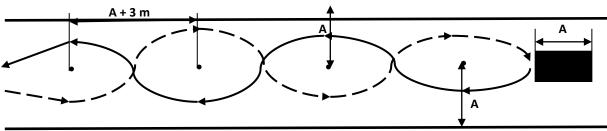
The automobile should move making a forward motion between the points and do it again but making a reverse motion.
