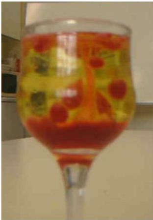
When you add the fizzing tablet in the mixture, it sinks to the bottom and then starts to dissolve. As it dissolves, it reacts with the water to make tiny bubbles of carbon dioxide, which is a gas. These bubbles attach themselves to blobs of coloured water and cause them to float to the surface. When the bubbles pop, the carbon dioxide gas escapes and the colour blobs sink back to the bottom of the bottle, and the whole thing starts over until the tablet is used up.
