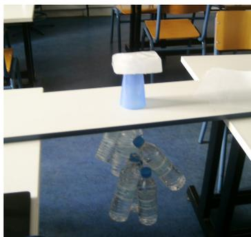
four bottles tied to each end on a piece of ice. After some time, it seems as if the fishing line is phasing through the piece of ice!
